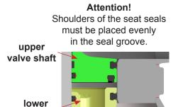
**3.1.** Press a short piece part of the seal into the groove.
